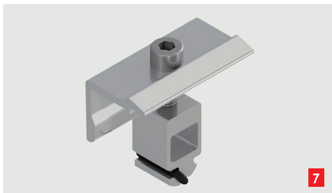
Universal end clip with cylinder head screw M8 for module heights of 30–40 mm or 41–46 mm for high support
