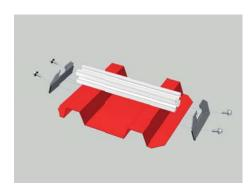
The profile rail is placed on the ribbing and aligned and then the sheet metal is inserted and bolted in place.
