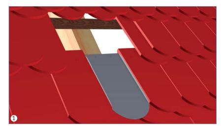
Remove the plain tile, where the roof hook will be placed, and also surrounding tiles.
