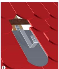
The plain tile roof hook will be fixed on the plate with 2 wood screws M8 × 100 and fastened through the roof board in the rafter.
