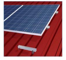
During the assembly you need to ensure that the trapezoidal sheet fasteners with the EPDM tape lies on the pleat surface and pressed down against the rail.
