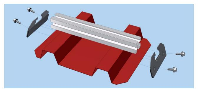
First align the tracks on the pleats of the trapezoidal roof. We recommend sticking the EPDM tape (two  $40 \times 30 \times 3$ ) onto the track area to seal the surface. The fasteners with EPDM tape are hooked into the side grooves of the track and pushed towards the pleat of the corrugated metal.
